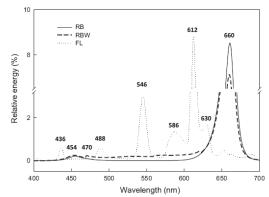
Fig. 3: Spectral distributions in the relative energy of the LED's and fluorescent Lamp.
